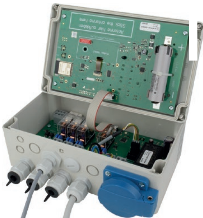
Figure 3: K-Pilot 2.4 control unit opened
