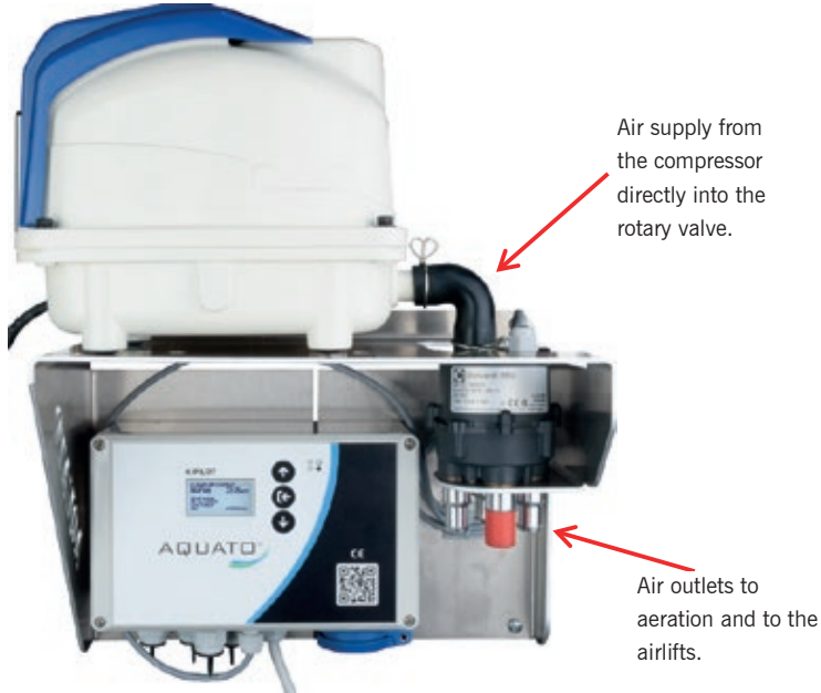
Figure 5: K-Pilot 2.4 control unit – air connections.
